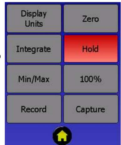
**14F. 100%:** Records the baseline value for 100%. This does not impact the display. To readout in percentage you must use the display units button to select percentage.
