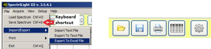
The spectrum data displayed in the main graph can be saved in binary format with file extension \*.ilt using “*Save Spectrum*”. You can load the saved binary file by clicking “*Load Spectrum*” and the loaded data will be displayed and replace the current spectrum.
