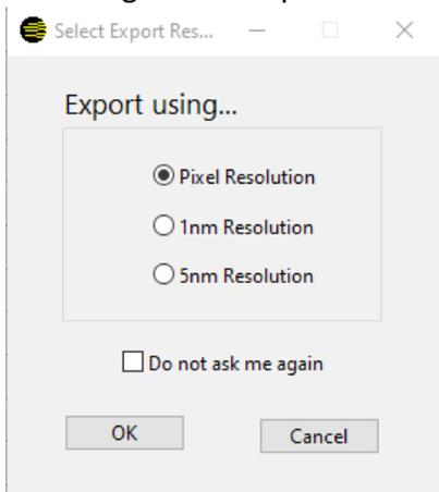
Checking “Do not ask me again”, the export routine will remember the resolution selection and the above pop-up window will not launch again. The default setting can be restored using Help\ Reset Factory Defaults.
