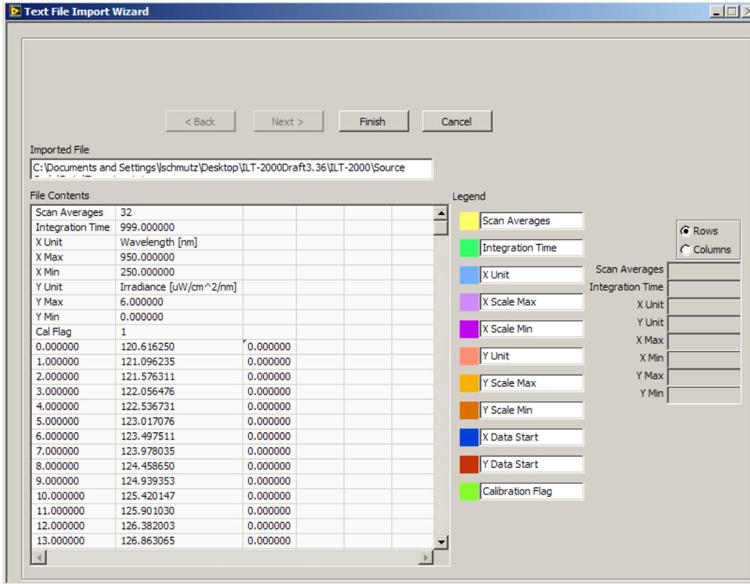
The data can be exported as .txt (“Export to Text File”) or .xls (“Export to Excel File”) using wavelength data in pixel resolution, in 1 nm or 5nm increments.
