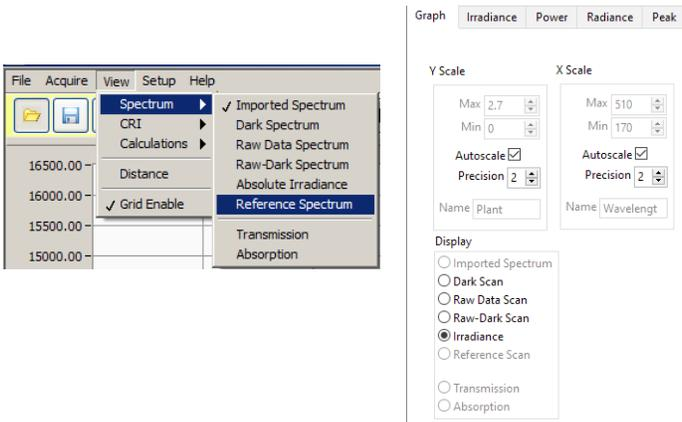
The user can choose to view different spectrum on the main graph area either from “View/Spectrum” menu or radio buttons in the “Display” section on the “Graph” tab page at the right side of the main GUI. For example the calibrated measurement results are displayed when checking the “Absolute Irradiance” menu or selecting “Irradiance” radio button. In T/A mode, the ratio spectrum can be displayed in percentage or logarithm scale when “transmission” or “absorption” checked.
