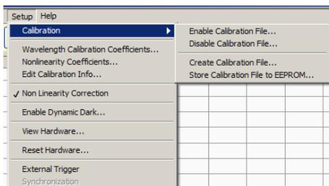
Under “*Calibration*” menu, the user can load and remove the calibration file with “*Enable Calibration File...*” or “*Disable Calibration File...*”. The “*Create Calibration File...*” and “*Store Calibration File to EEPROM...*” are normally reserved for use by International Light Technologies and can not be accessed without a password.
