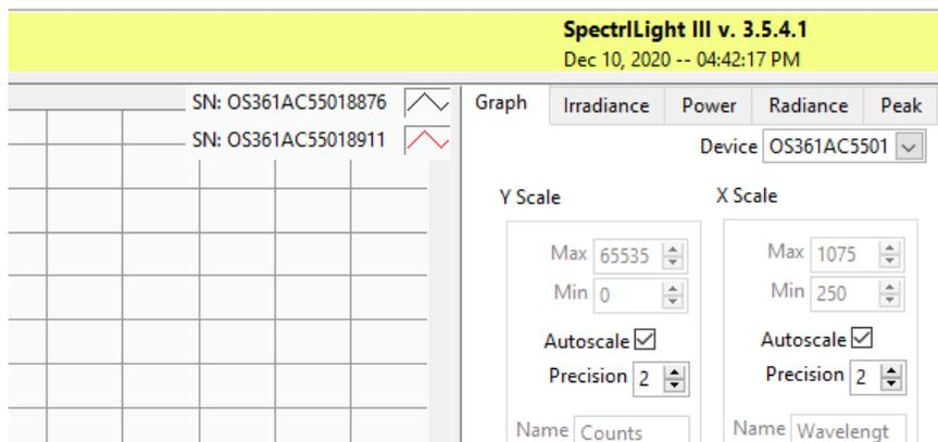
The process of selecting the calibration file for the spectrometer is the same as while using a single spectrometer, except the file has to be chosen using a pop-up window as shown below for each spectrometer. The process of acquisition is the same as for a single spectrometer. Scans for all the spectrometers are also displayed and saved together.
