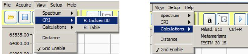
The calculated color rendering index can be seen from the pop up window through the “CRI” menu. The rendering index values are tabulated for 15 different color test samples with reference to black body illuminant with the same measured CCT “Ri Indices BB”, an Illuminant A at 2856K and a D65 lamp at 6500K “Ri Table”.
