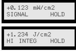
'HOLD': This message will blink in the 'status' register (lower right corner of the LCD) after the 'HOLD' button has been pressed, activating the 'HOLD' feature. The most recent reading will be frozen on the data display. To remove the 'HOLD' status, toggle the 'HOLD' button again or hit a function key ('SIGNAL', 'INTEGRATE', or 'ZERO') to select a new mode of operation.
