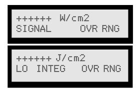
'OVR RNG': This message will blink in the 'status' register (lower right corner of the LCD) when the input detector signal exceeds the measurement range of the system. In addition, plus signs take the place of numerals in the data display, so that the top line will read '+++++  $\pm$  W/
