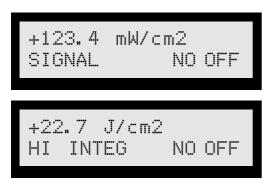
'NO OFF': This message will blink in the 'status' register (lower right corner of the LCD) when the automati c 10 minute shutoff feature has been disabled. This indicates that a previous user selected 'AUTO SHUT OFF' 'DISABLED' using the programming mode capabilities.
