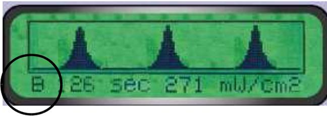
The **baseline profile** shows all three Lamps having a uniform output of 271mW/cm<sup>2</sup>
